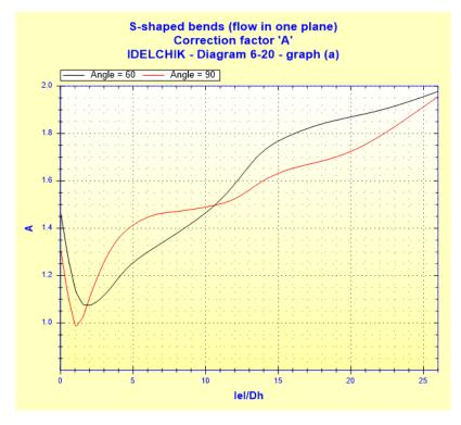
Total pressure loss coefficient (based on the mean velocity in the bends):
