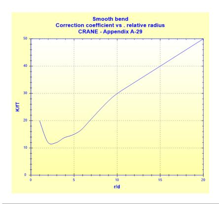
Total pressure loss coefficient (based on mean velocity in helical tube):
