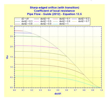
Total pressure loss coefficient (based on the major pipe velocity):
