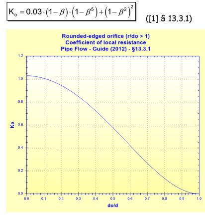
Total pressure loss coefficient (based on the mean pipe velocity):
