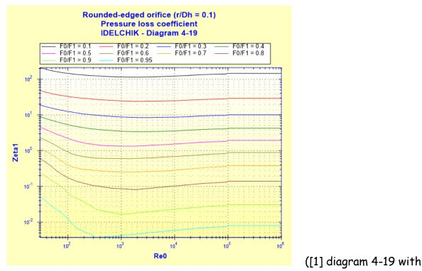
Pressure loss coefficient (based on the mean pipe velocity):
