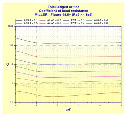
Total pressure loss coefficient (based on mean velocity in pipe):
