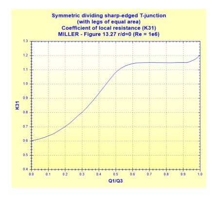
Pressure loss coefficient of the right branch (based on mean velocity in the common branch):
