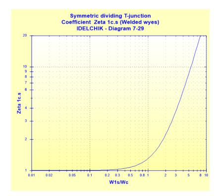
Pressure loss coefficient of the left branch (based on mean velocity in the common branch):
