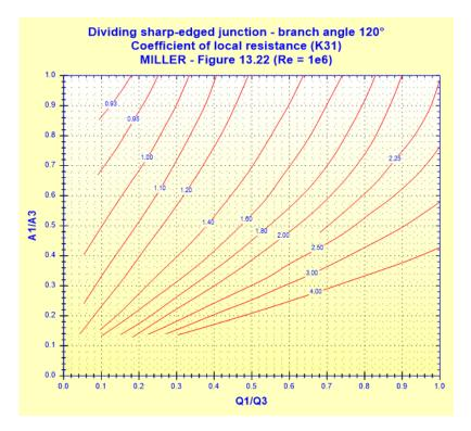
For any angles between 45 ° and 120 °, the coefficient  $K_{31}$  is obtained by linear interpolation between the values of  $K_{31}$  calculated at 45 °, 60 °, 90 ° and 120 °.
