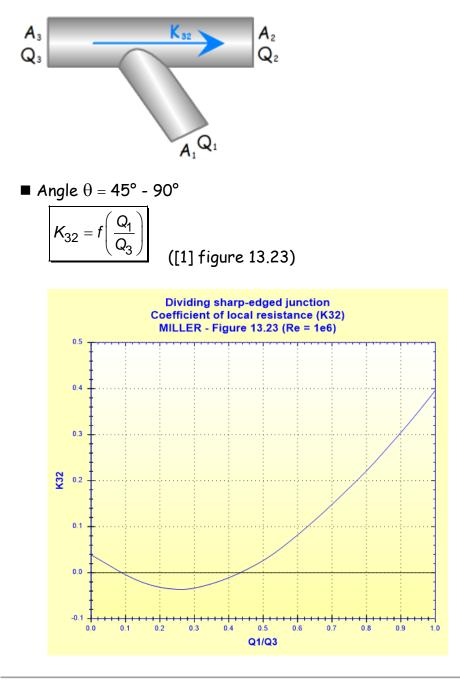
Pressure loss in the lateral branch (Pa):
