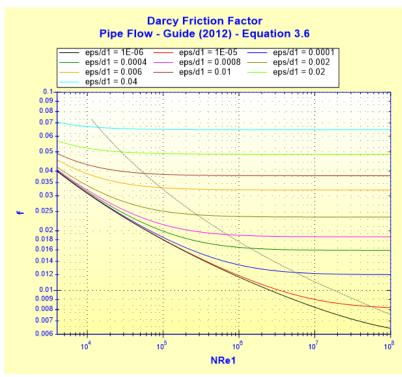
Friction pressure loss coefficient:
