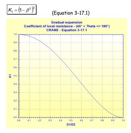
Total pressure loss coefficient (based on mean velocity in minor diameter):
