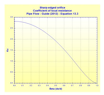
Total pressure loss coefficient (based on the mean pipe velocity):
