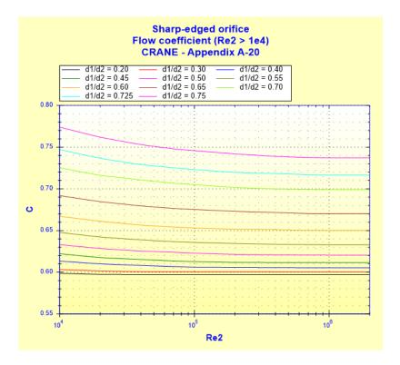
Resistance coefficient of orifice:
