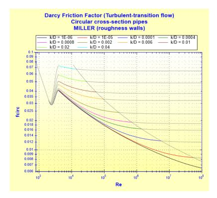
Complete turbulence region Darcy Friction Factor (Turbulent-quadratic flow) **Circular cross-section pipes** MILLER (roughness walls) k/D = 1E-06 k/D = 1E-05 k/D = 0.0001 - k/D = 0.0004 k/D = 0.0008 k/D = 0.002 k/D = 0.04 k/D = 0.006 — k/D = 0.01 \_ k/D = 0.020.1 0.09 .... 0.08 0.07 0.06 0.05 0.04 0.035 0.03 fcirc 0.025 0.02 0.018 0.016 0.014 0.012 0.01 0.009 0.008 0.007 0.006 10<sup>4</sup> 10<sup>6</sup> 10<sup>3</sup> 10<sup>5</sup> 10 10 Re
