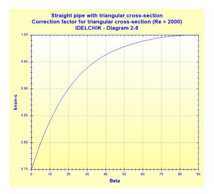
Darcy friction factor for triangular cross-section:
