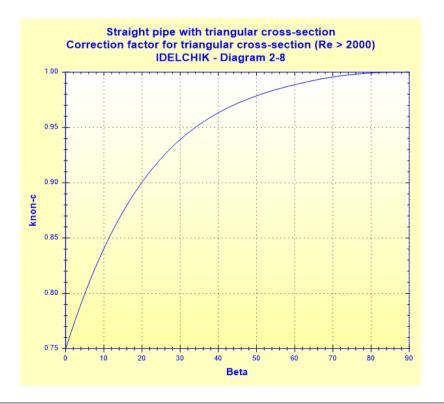
Darcy friction factor for triangular cross-section:
