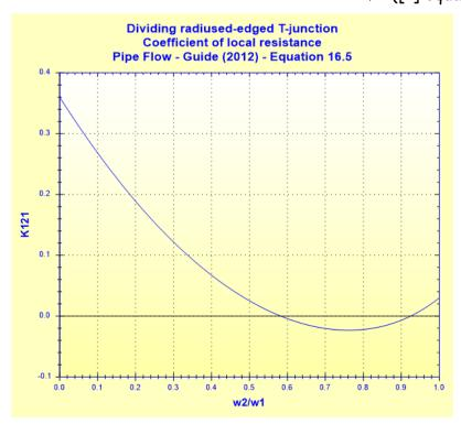
Coefficient based on mean velocity in the straight branch:
