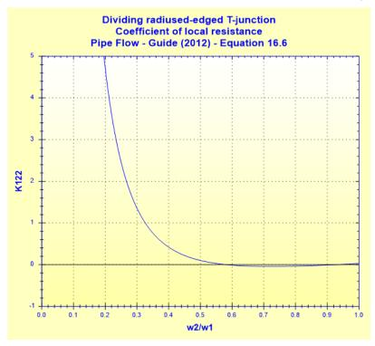
Pressure loss coefficient of the side branch:
