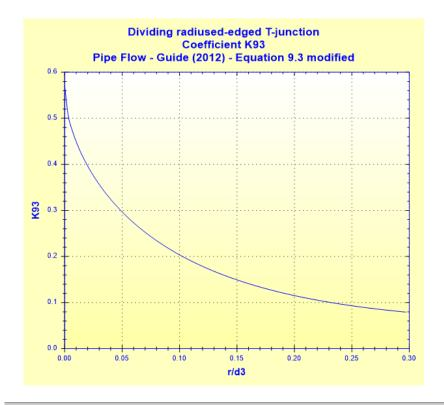
Pressure loss coefficient of the straight branch:
