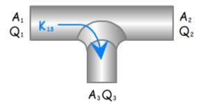
Coefficient based on mean velocity in the common branch:
