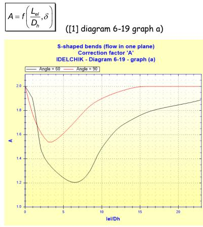
Total pressure loss coefficient (based on the mean velocity in the bends):
