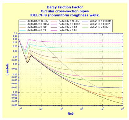
Pressure loss coefficient (based on the mean pipe velocity):
