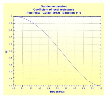
Total pressure loss coefficient (based on mean velocity in minor diameter):
