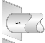
Sharp-edged entrance mounted at a distance
