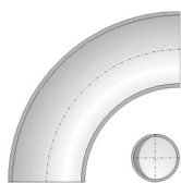
Smooth bend with circular cross-section
