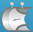
Nozzle and Venturi nozzle flowmeter
